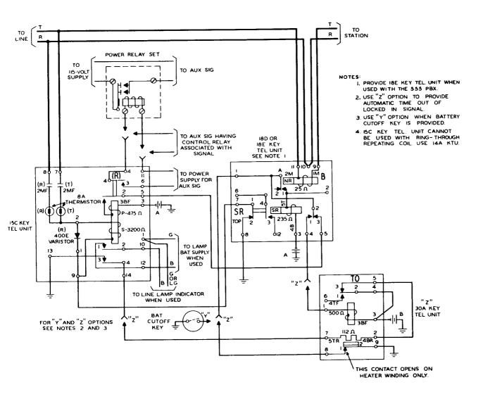
Fig. 8 - Connections and Circuit Operation for Continuous Auxiliary Signals
