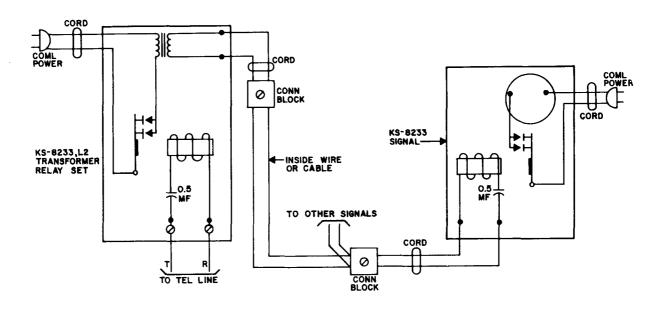
Fig. 4 - KS-8233, L2 Transformer Relay Set
