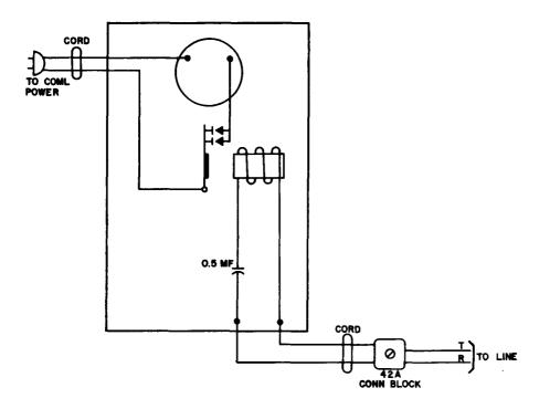
Fig. 2 - Typical Relay Equipped Signal
