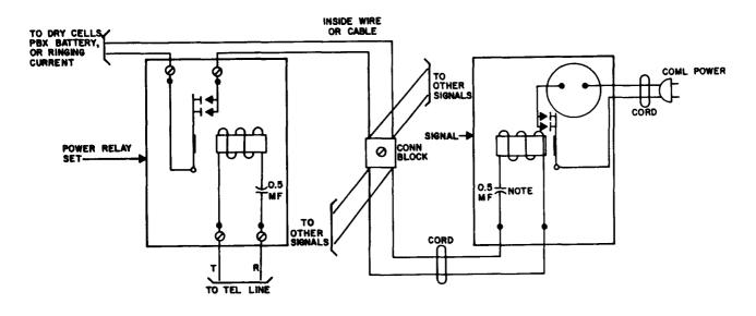
MOTE: SIGNALS DESIGNED FOR USE WITH OC DO NOT CONTAIN & CAPACITOR.
