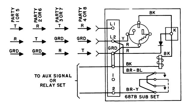
Fig. 6 - Auxiliary Signals on Party Lines
